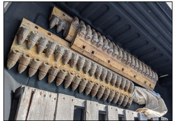
Carbide-tipped grader blades are recommended for grading DSA.
